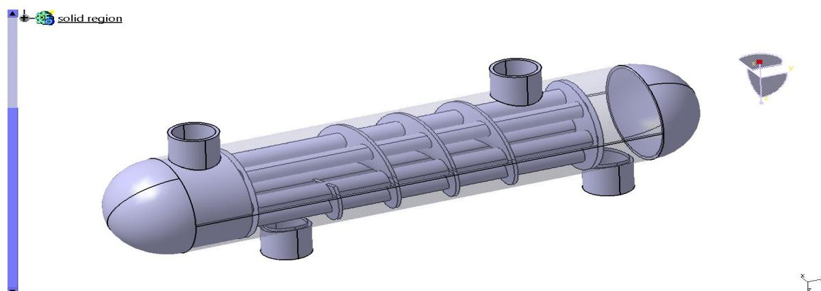
**6.1 3D Modeling of shell and Tube heat Exchanger (CATIA)**
