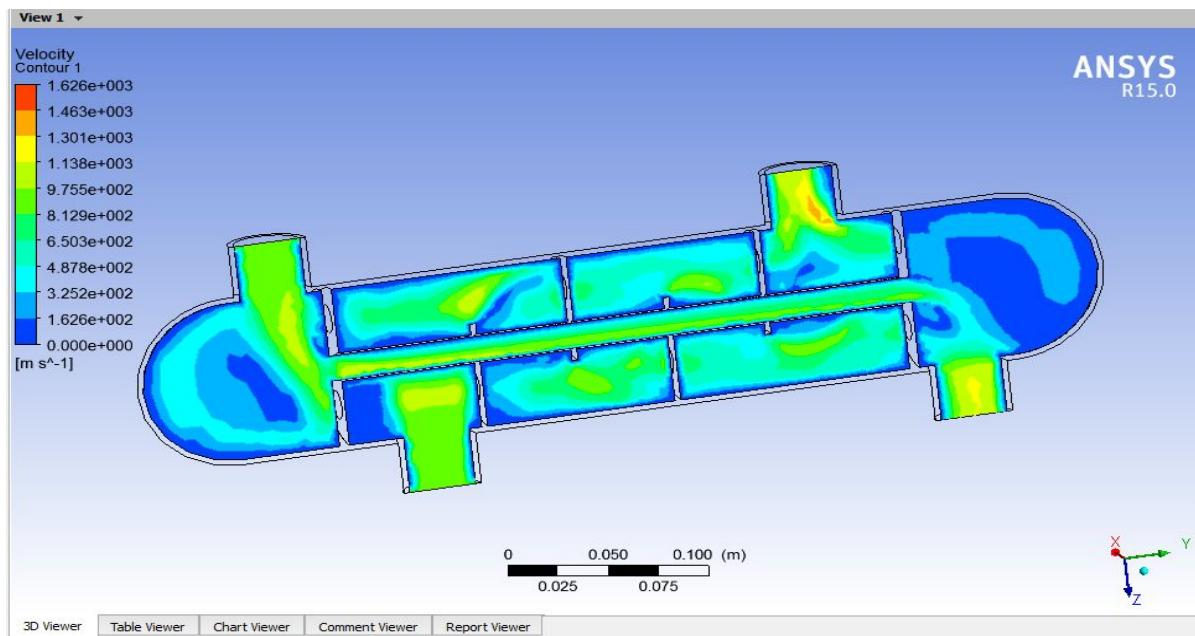
**Figure 7.10 vertical velocity Distribution across the tube and shell**
