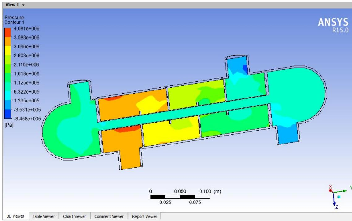
**Figure 7.8 vertical baffle -Pressure Distribution across the shell and tube**
