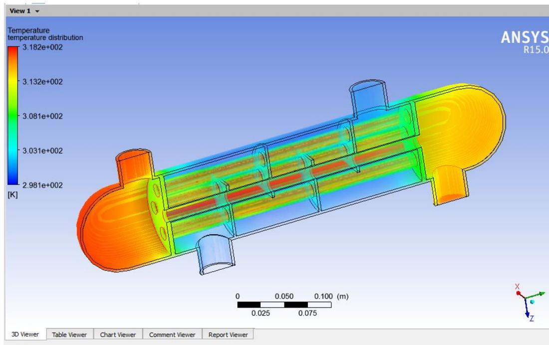
**Figure 7.5 Vertical baffle Temperature Distribution across the tube and shell (volume transperant)**
