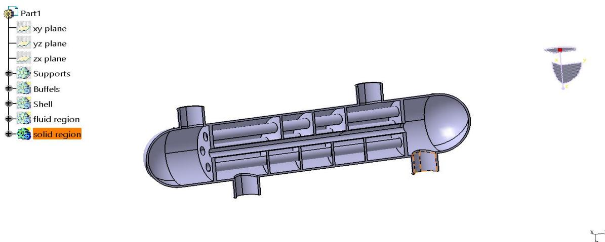
**6.2 3D Modeling sectional view of shell and Tube heat Exchanger (CATIA)**
