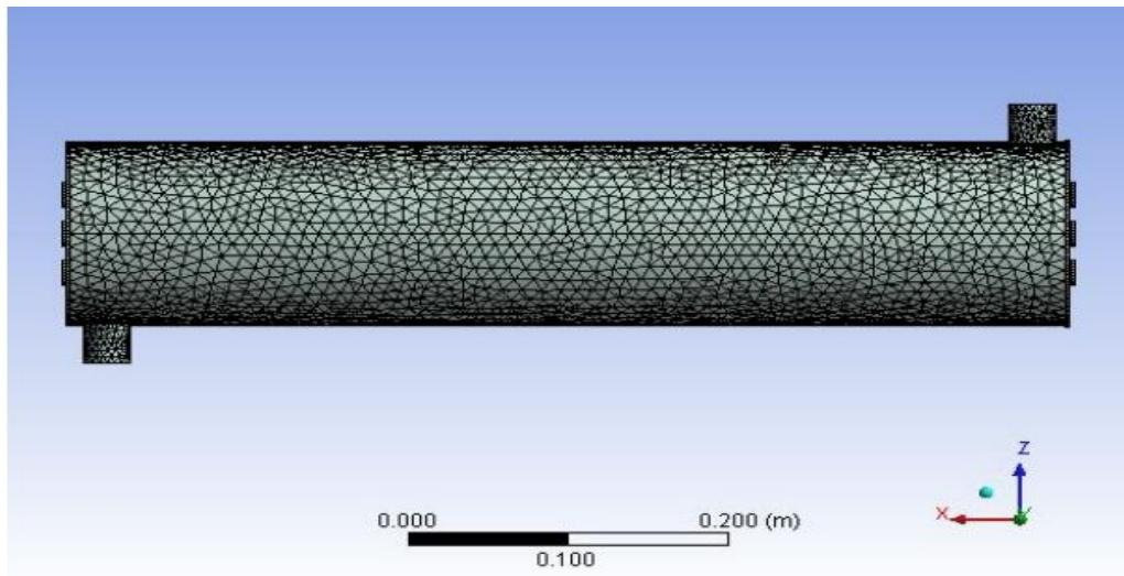
**Fig 7.2 Meshing diagram of shell and tube heat exchanger**
