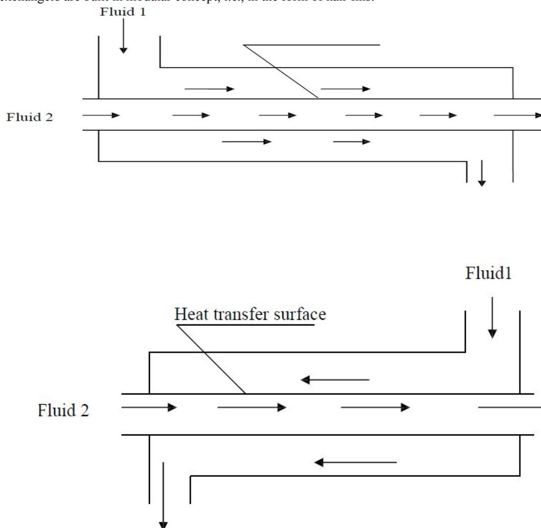
*Fig 1.3: Double pipe heat exchanger*
