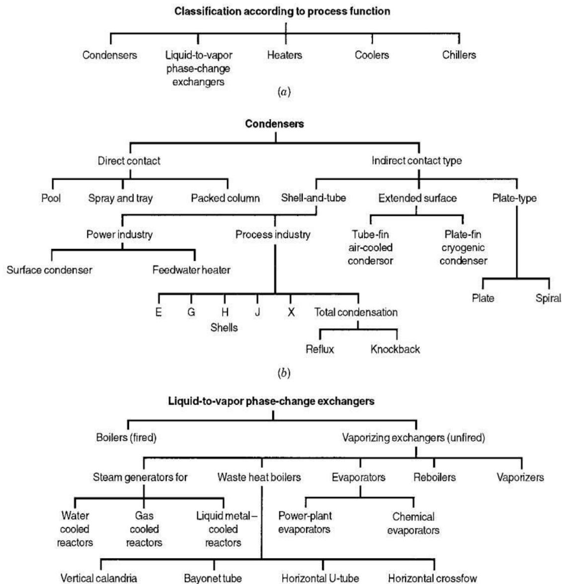
**Fig 1.2 Classification of heat exchangers**
