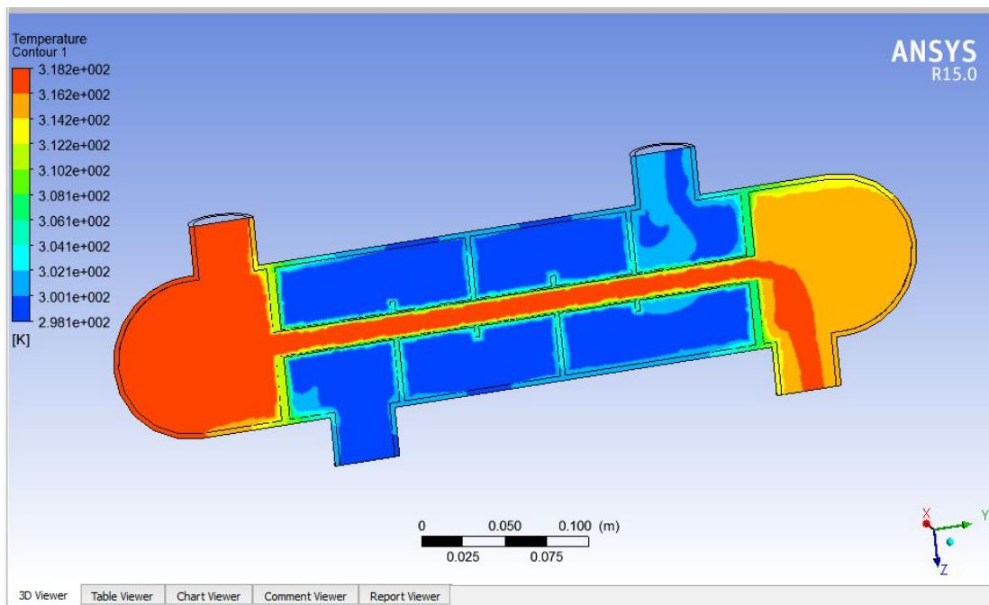
**Figure 7.4 Vertical baffle Temperature Distribution across the tube and shell**
