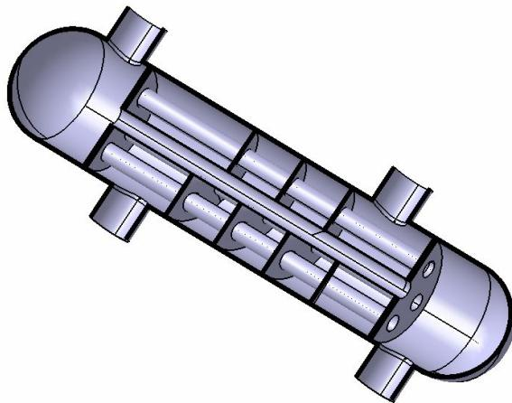
**Fig 7.1 Isometric view of arrangement of baffles and tubes of shell and tube heat exchanger with baffle inclination**
