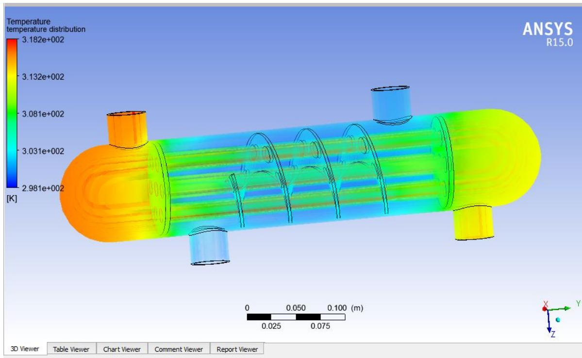
**Figure 7.7 Helical baffle Temperature Distribution across the tube and shell (volume transperant).**
