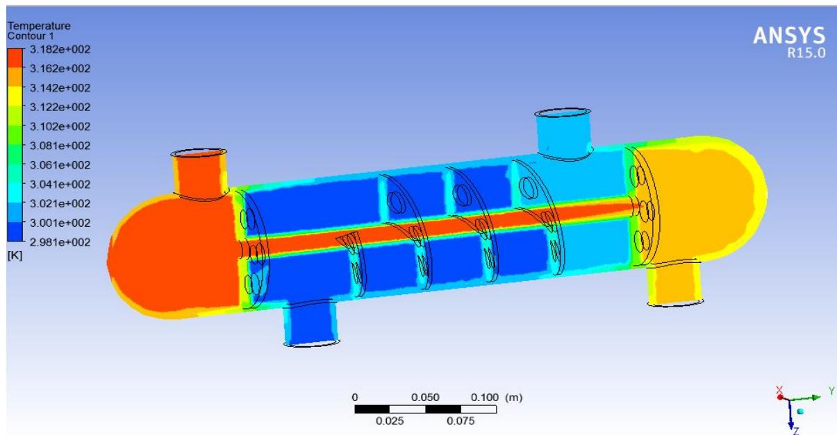
**Figure 7.6 helical baffle Temperature Distribution across the tube and shell**
