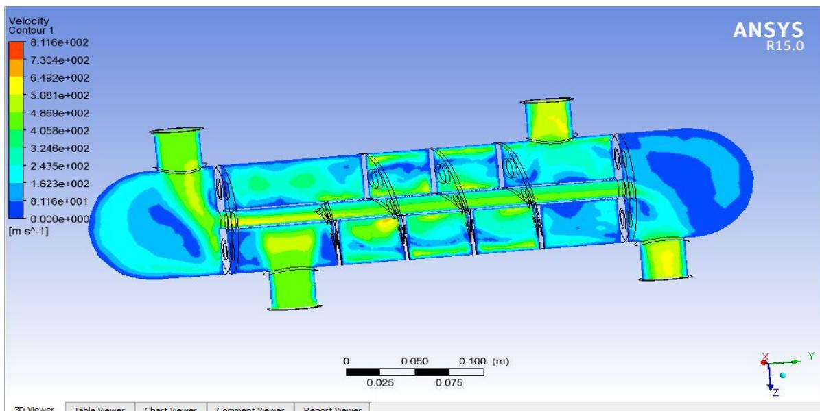
**Figure 7.11 helical baffle velocity Distribution across the tube and shell**
