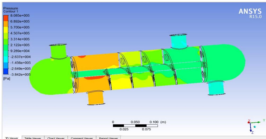
**Figure 7.9 Helical baffle Pressure Distribution across the tube and shell**
