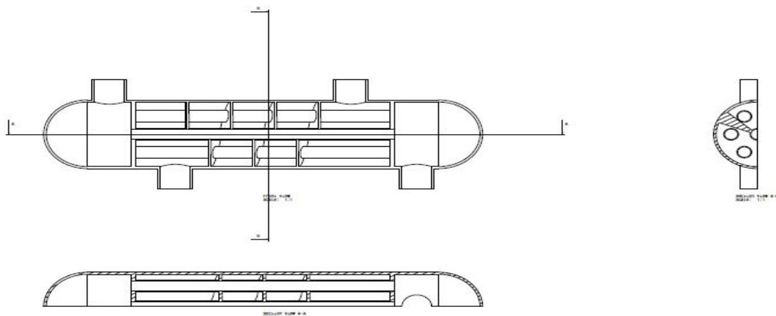
**6.4 2D orthographic sectional views of shell and Tube heat Exchanger (CATIA)**
